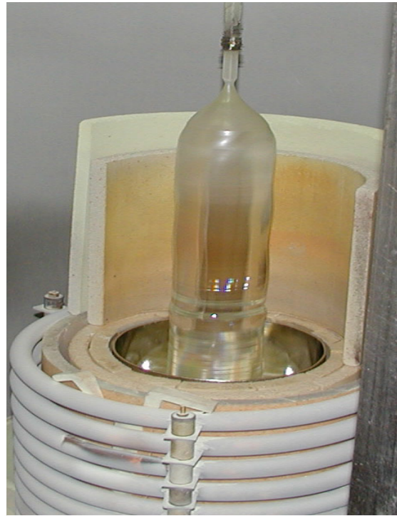
PbWO 4 crystal grown in ingot
