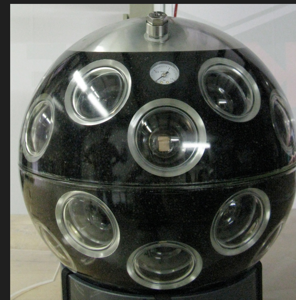
Multi-PMT digital optical module (“DOM”)
