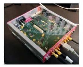
SAMPIC 1.5 GHz bandwidth 10 Gs/s (used at 6.4 Gs/s 11 bit 64 samples 16 channels Maximum rate ~500 kHz)
