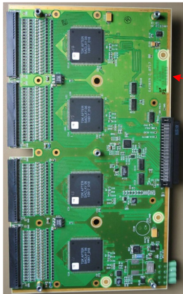
T2K FEC: 4 AFTER chips 288-channels
