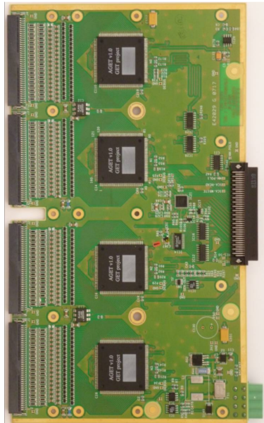
MINOS FEC: 4 AGET chips (pin-compatible with AFTER) 256-channels
