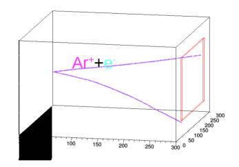
The electron and positron travel through the gas (mostly Argon) and ionises it, freeing many electrons and positive ions This takes a few nanoseconds
