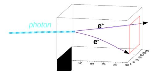
The incoming photon interacts with the gas and decays into an electron-positron pair
