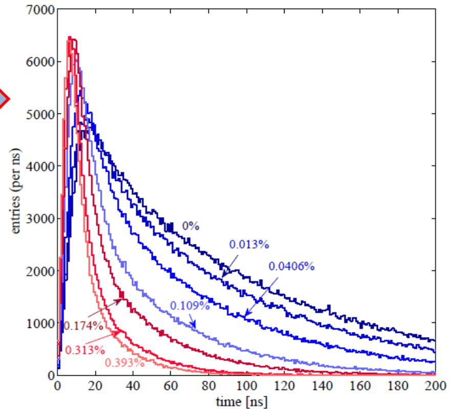
scintillation in Xe/CH<sub>4</sub> admixtures (P=1.27bar)
