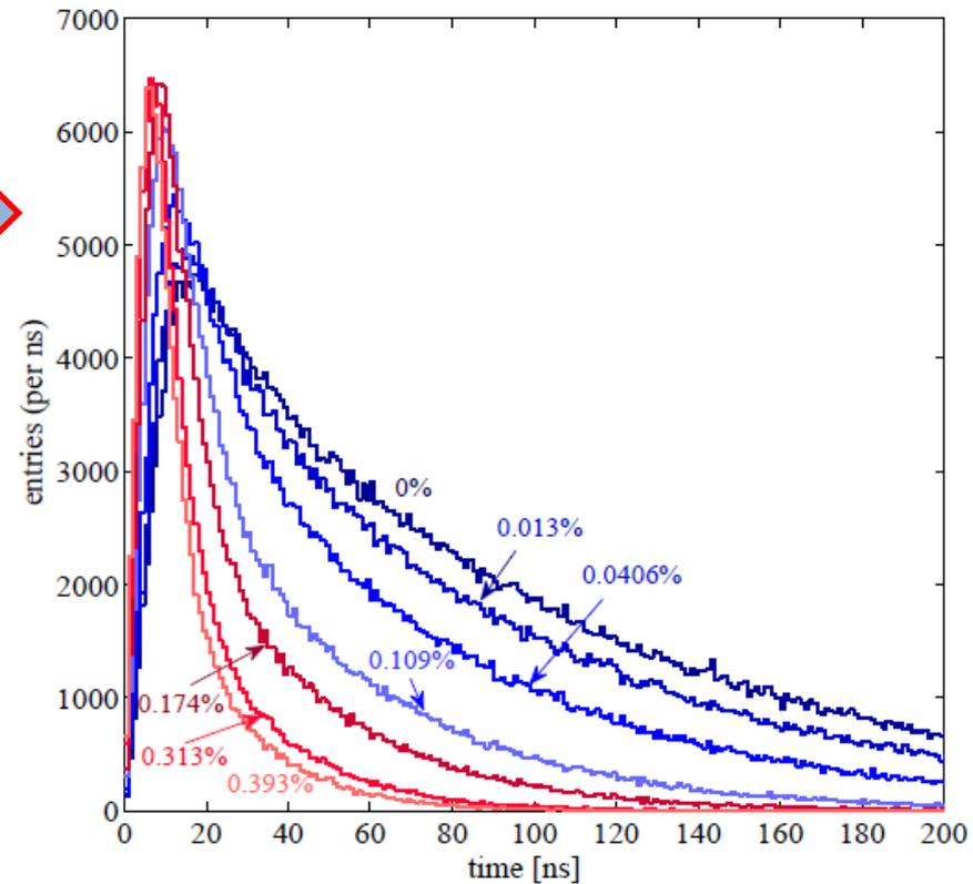
scintillation in Xe/CH<sub>4</sub> admixtures (P=1.27bar)
