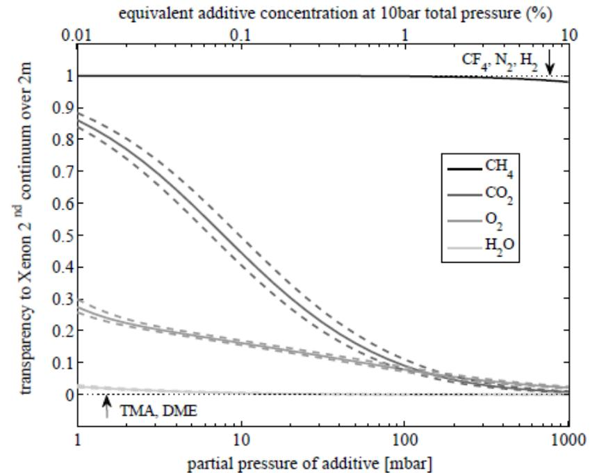
Fig. 2. Estimated transparency to scintillation from Xenon 2<sup>nd</sup> continuum as a function of partial pressure of the additive, over a 2 meter-long TPC. Dashed lines are obtained assuming 20% errors in the cross-sections.
