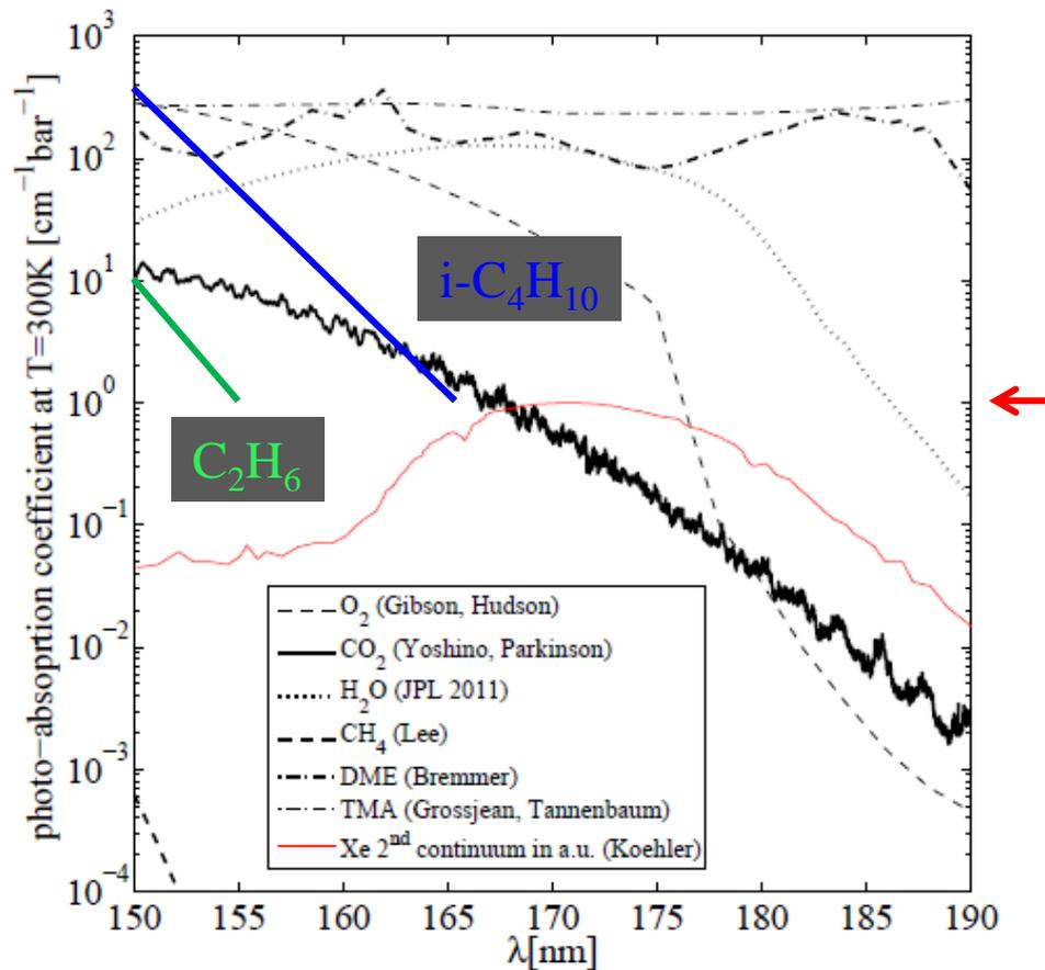
Fig. 1. Compilation of photo-absorption coefficients of some relevant TPC admixtures at around  $T = 300\text{K}$  in the region corresponding to the Xenon 2<sup>nd</sup> continuum, [9–18]. The reference spectrum from Koehler has been overlaid as a thin continuous line [2]. For  $\text{H}_2$ ,  $\text{N}_2$  and  $\text{CF}_4$  there is no data in the region shown, and their cross-sections are plausibly orders of magnitude below that of  $\text{CH}_4$ .
