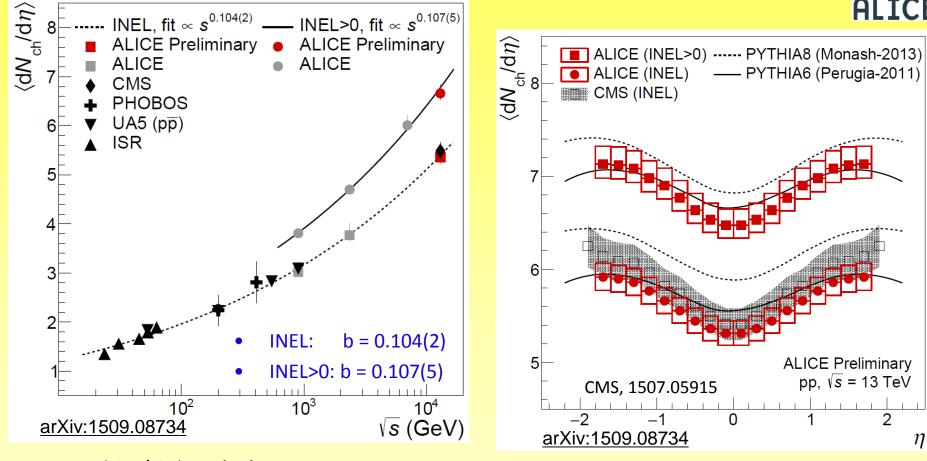
INEL:  $\langle dN/d\eta \rangle$  in  $|\eta| < 0.5$
