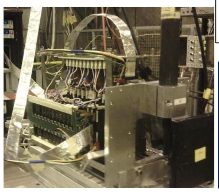
19-Layer full set used in SPS Beam-Line with Tungsten plates, Silicon sensors, associated electronics etc
