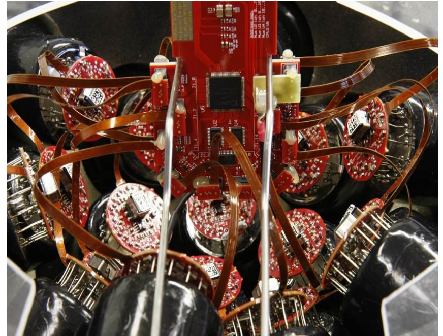
Electronics to read out the photomultiplier tubes and calibration instrumentation inside the KM3NeT DOM
