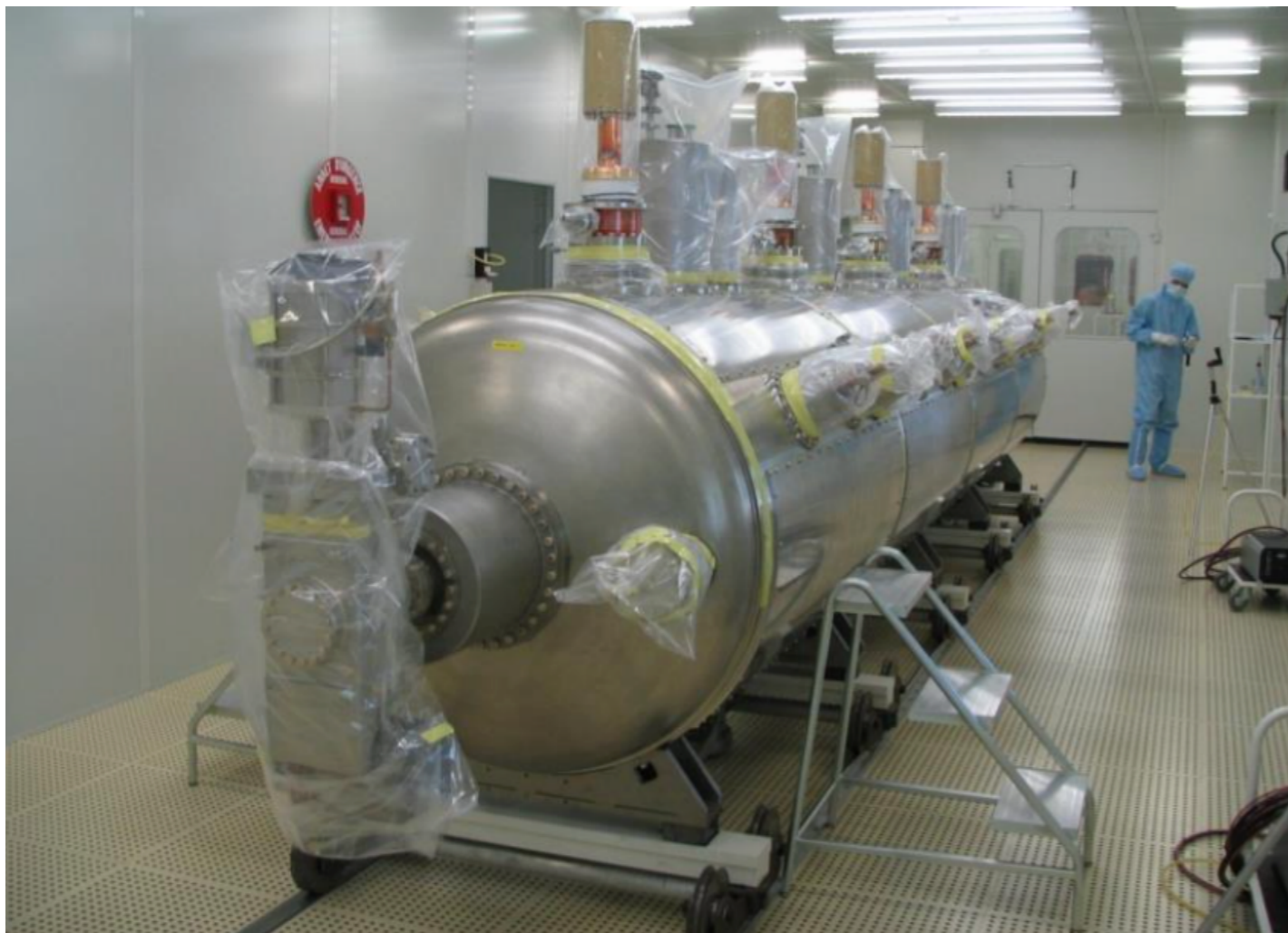
LHC Cryomodule on SM18 cleanroom rail system
