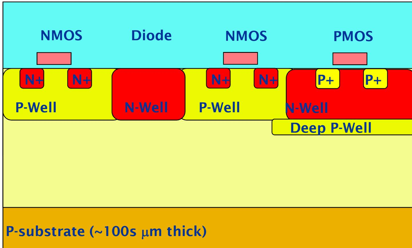
*Standard CMOS with additional deep P-well implant. Quadruple well technology.*
