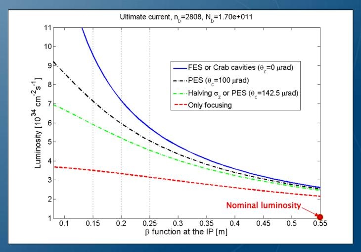
The D0 gives the opportunity of gaining in luminosity with a lower increase in the beam current by modifying the geometry of the collision to take full (or almost full) advantage of the decrease of the  $\Omega^*$ .
