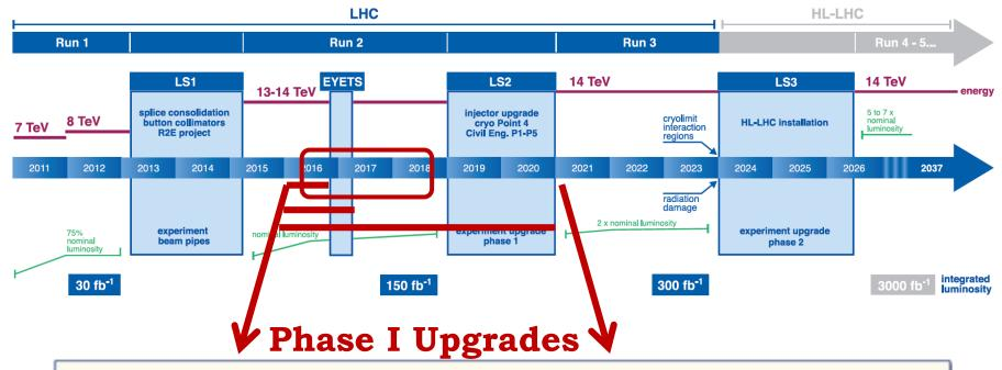
Phase 1 upgrades: Prepare for 1.6 x  $10^{34}$  Hz/cm<sup>2</sup>, <PU> ~40,  $\leq$  200 fb<sup>-1</sup> by LS2 Prepare for 2.5 x  $10^{34}$  Hz/cm<sup>2</sup>, <PU> ~ 60,  $\leq$  500 fb<sup>-1</sup> by LS3
