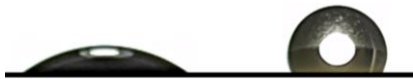
Figure 1 The characteristics of droplets are plano convex surfaces on the hydrophilic and hydrophobic surfaces.
