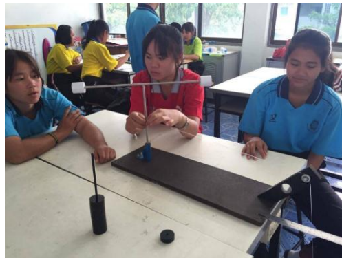
Figure 2 The real set up of the experiment for moment of inertia.
