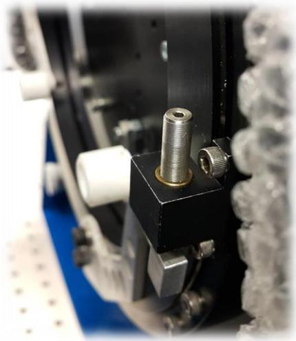
The optical flats were mounted on the three-point type mounting. It should be noted that the mounting can be adjusted the clamping force by the screw, pitch distance of 0.7 mm
