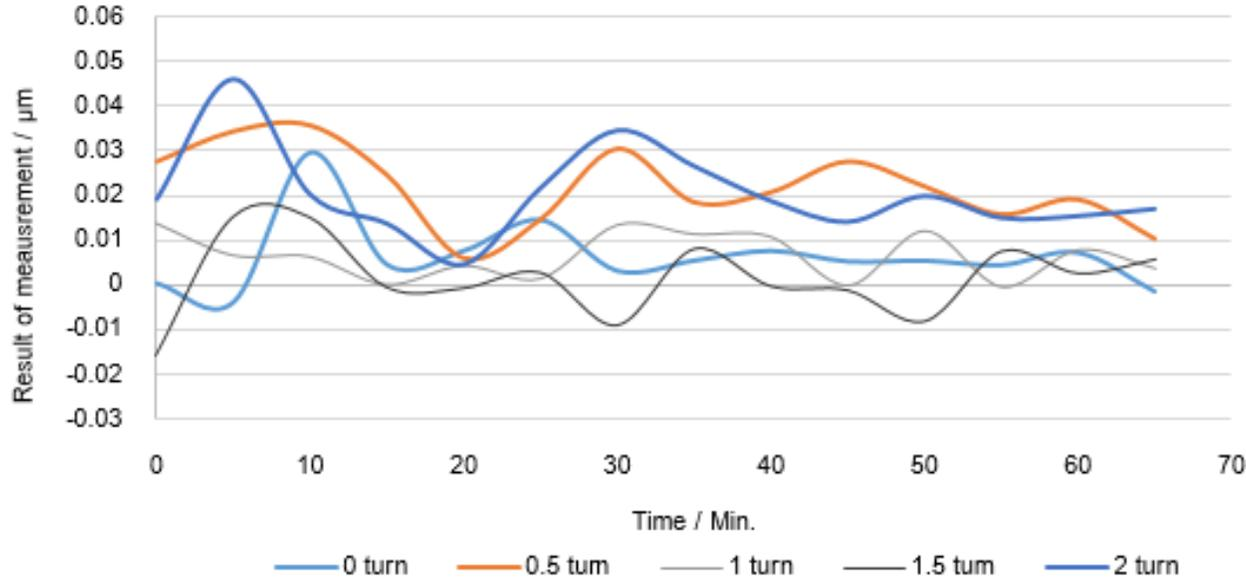
Result when the optical flat mounted on the three-point type mounting with increasing clamping force. The harder clamping force is, the large variation in flatness observed. The clamping force may result to deformation of the optical flat.
