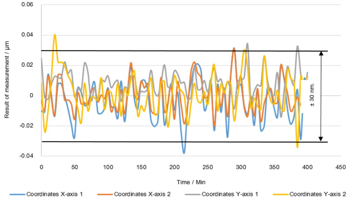
The variation is well within  $\pm 30 \text{ nm}$ . It should be noted that the measurement uncertainty of the flatness interferometer is  $\pm 31.65 \text{ nm}$ . Thus, we can conclude that the variation of  $\pm 30 \text{ nm}$  can be due to environment and it is well within the measurement uncertainty.
