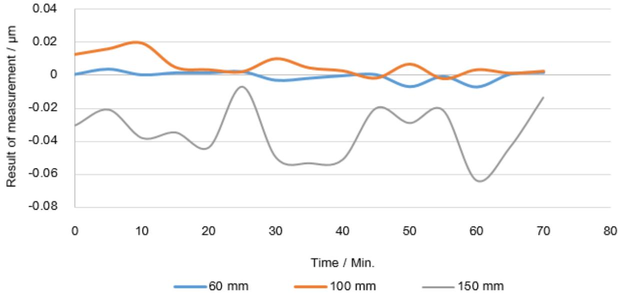
Variation in height at point  $Y_1$  of optical flat A, B, and C
