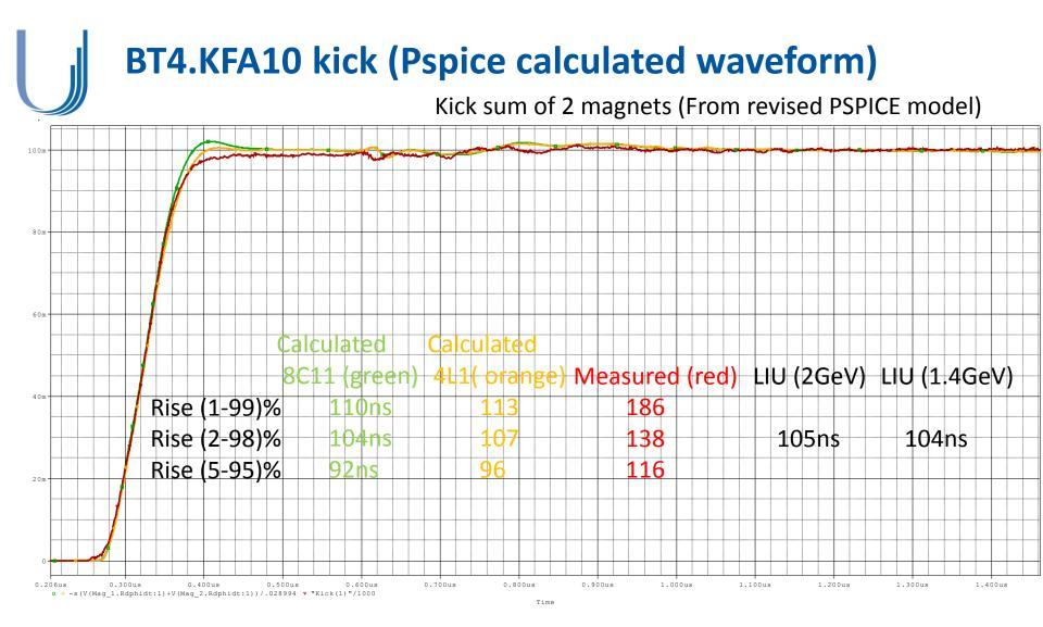
The actual ferrite grade is assumed to be 4L1. (must be replaced by 8C11) Cable impedances are not exactly  $25\Omega$ . (variations from 24.8 to 25.5 for PFLs and Transmissions explain reflections)
