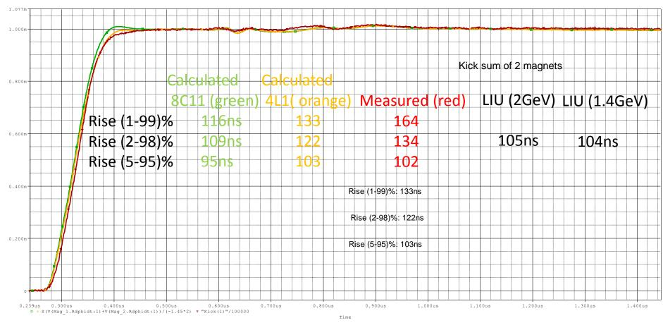
The actual ferrite grade is assumed to be 4L1. (must be replaced by 8C11) Cable impedances are not exactly  $25\Omega$ . (variations from 24.8 to 25.5 for PFLs and Transmissions explain reflections)
