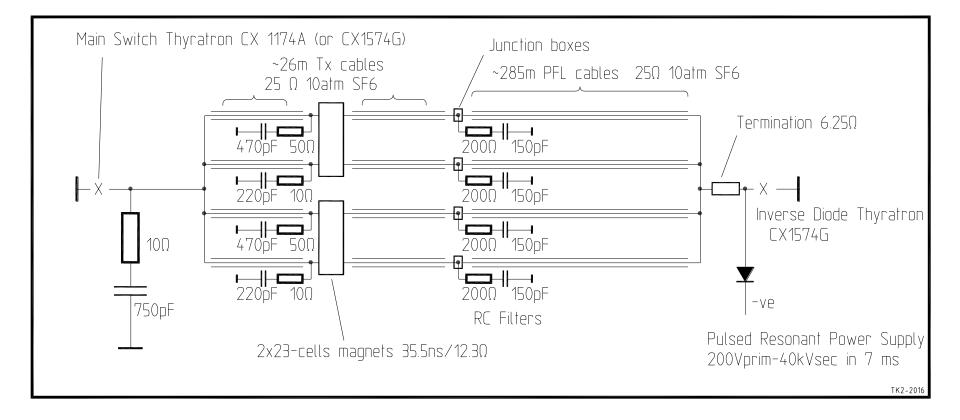
One generator supplying two magnets in parallel. Magnets equipped with CMD5005 ferrite blocks. Magnets are charged with the PFLs.
