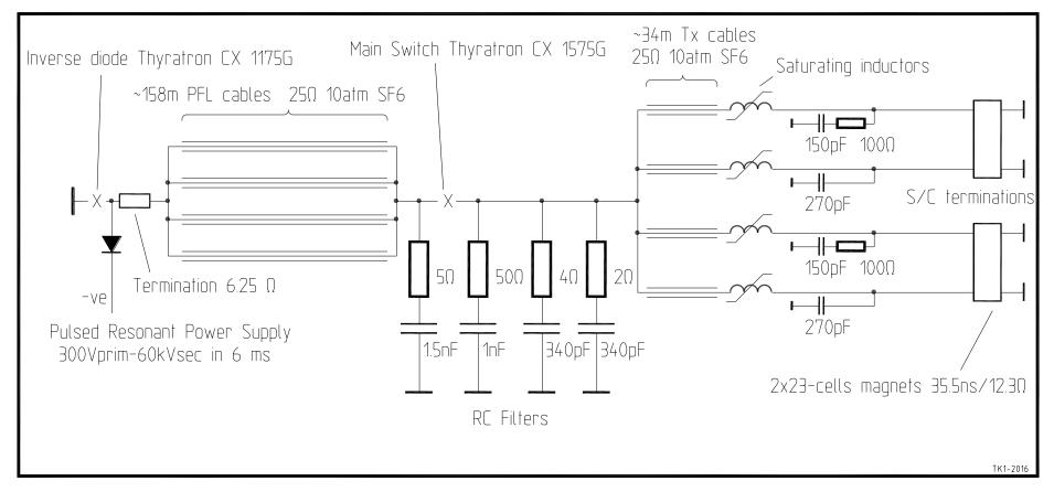
One generator supplying two magnets in parallel.
