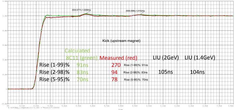
The present kick waveform complies with LIU specification without margin. The overshoot is not present in the measured waveforms. Cable impedances are not exactly 25Ω. (variations from 24.8 to 25.5 for PFLs and Transmissions explain the reflection bumps)
