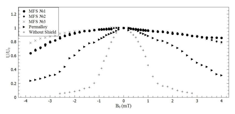
The relative amplitude of the PMT-85 output signal, for different types of shields, depending on the external magnetic field in the direction of the magnetic field perpendicular to the shield.
