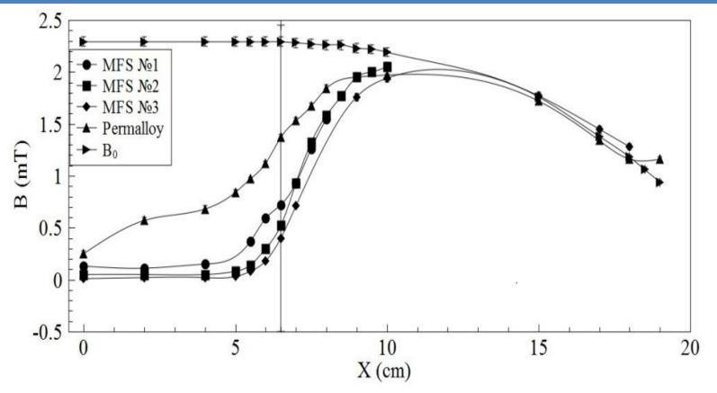
The distribution of the magnetic field along the longitudinal axis of the various shield's types. <u>O on the horizontal axis</u> corresponds to the middle of the longitudinal size of the shield. <u>The vertical line</u> is the end of the cylindrical shield. The magnetic field  $(B_0)$  is directed perpendicular to a longitudinal axis of the shield.
