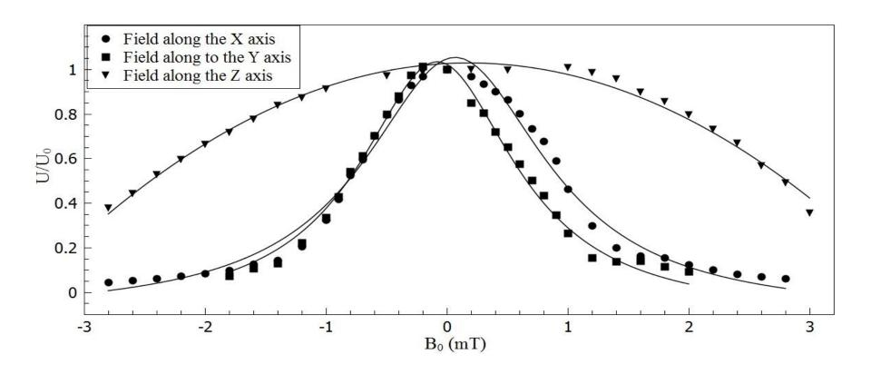
Dependence of the relative amplitude of the output signal of an unshielded PMT-85 on the magnetic field along the axes (X, Y) and parallel to the axis (Z).
