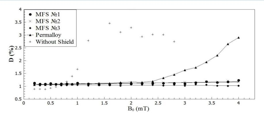
Dependence of the amplitude resolution of PMT-85 pulses on the induction of magnetic field without shield and also with shields of permalloy and MFS N 1 - N 3, with direction of the magnetic field perpendicular to the Z axis.
