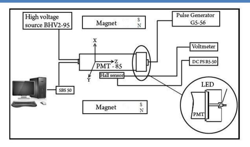
The scheme of experimental setup for the study of the screening effectiveness of PMT by different magnetic shields.
