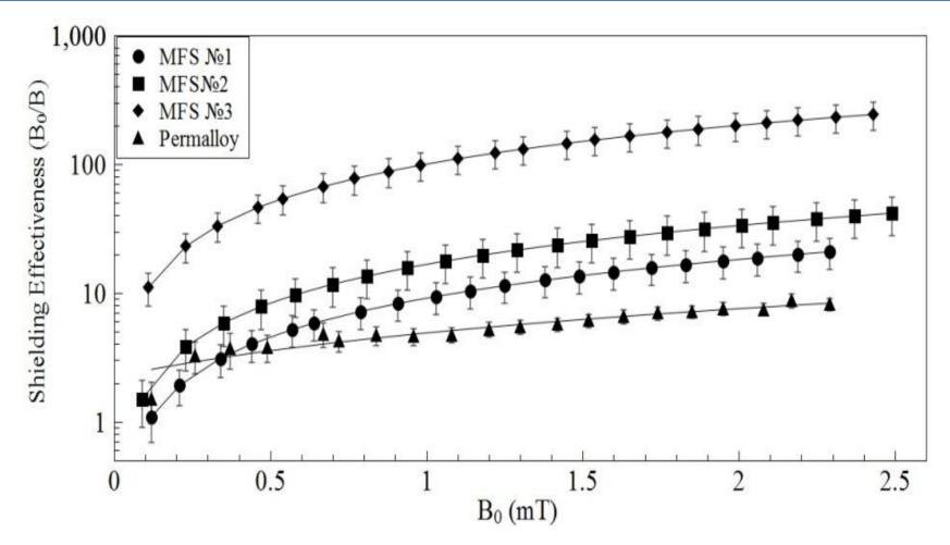
Shielding effectiveness of various shield's types (in the middle of the shield) depending on the value of the external magnetic field directed perpendicular to the longitudinal axis of the shield.
