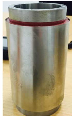
Rotor banding (done by Alxion)
