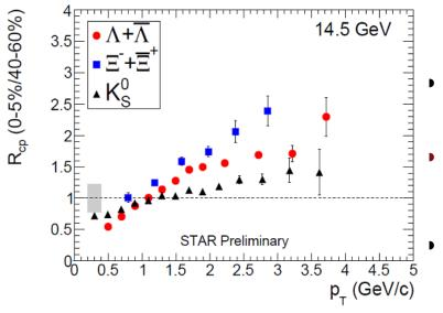
$$R_{\rm CP}(p_T) = \frac{[d^2\sigma/(N_{\rm bin}p_Tdp_Tdy)]_{\rm central}}{[d^2\sigma/(N_{\rm bin}p_Tdp_Tdy)]_{\rm peripheral}}$$
