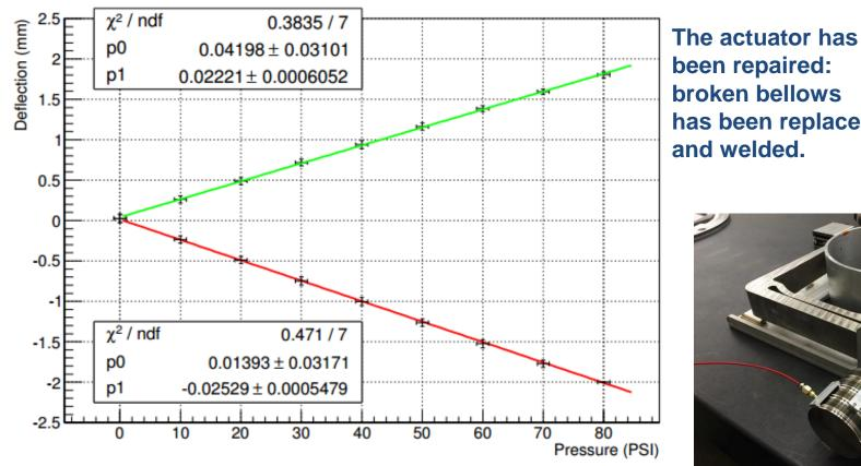
broken bellows has been replaced
