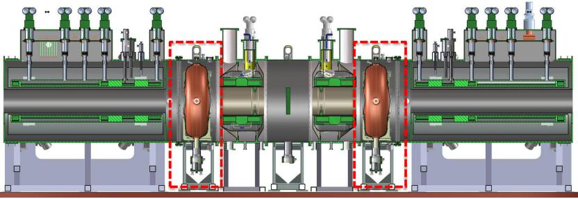
• MICE cooling channel needs two RF modules
