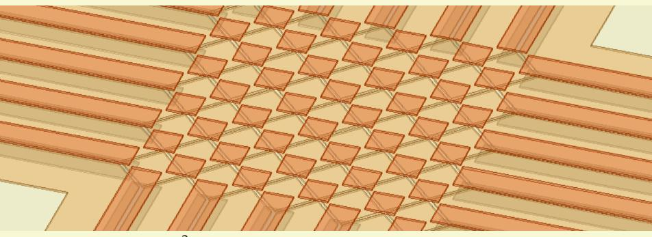
25 x 25 mm<sup>2</sup> C-DIR finite-element modelled with 8pF pattern capacitance
