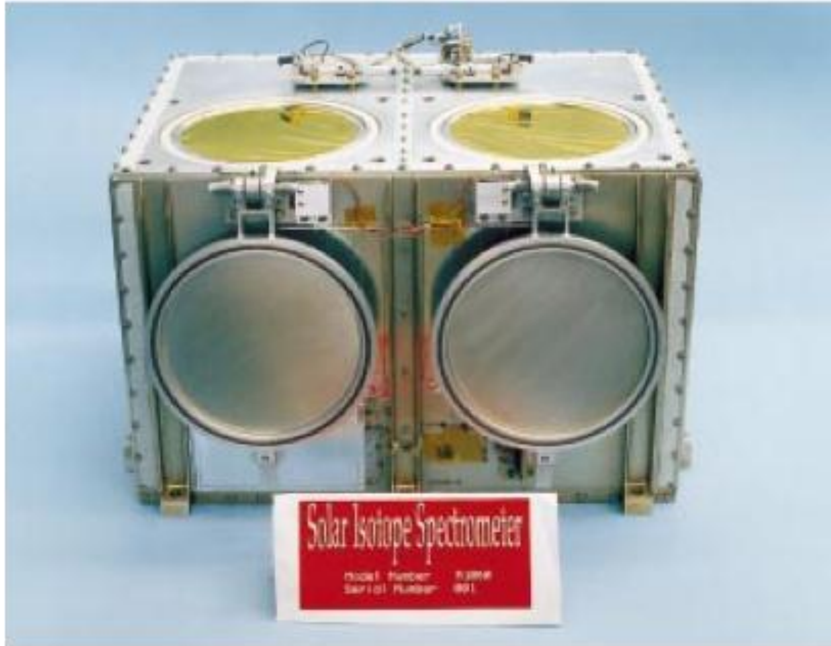
Figure 1. Photograph of the SIS instrument with the acoustic covers open. The dimensions of the housing are 30.0 \times 41.9 \times 27.5 cm.
