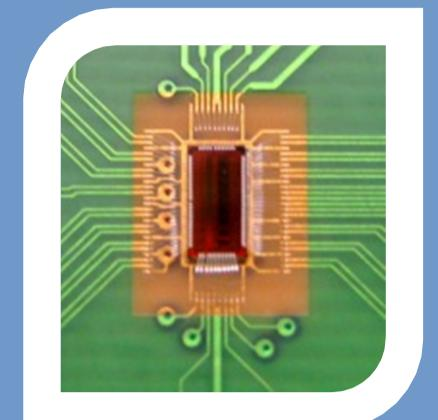
**High Performance Time-to-Digital Convertor** A programmable TDC developed
