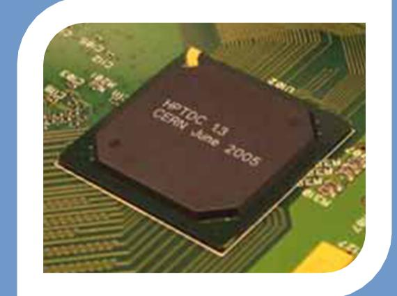
/discriminator developed at CERN. The time over threshold technique can provide pulse height.
