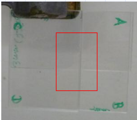
Four PMMA plates with thickness from 2-9 mm
