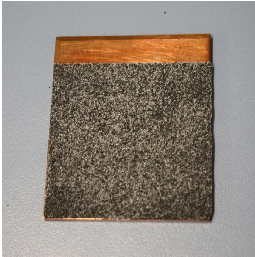
Simple oxide mixture on copper plate with carbon tape
