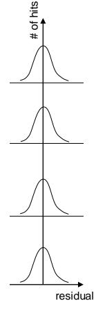
residual = distance between hit and the fitted track
