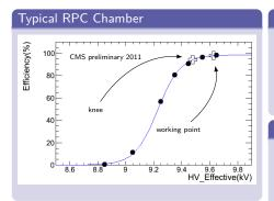
Fitted sigmoidal efficiency curve
