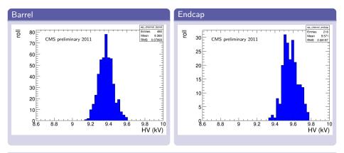
The difference between Barrel and Endcap RPCs comes from a difference in construction techniques A procedure of averaging is applied since different rolls share a High Voltage supply channel
