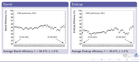
Average hit efficiency for Barrel and Endcap
