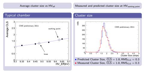
The cluster size is defined as the number of contiguous strips associated to a hit; on average it remains within specifications, i.e. below 2 strips (important for trigger algorithm)
