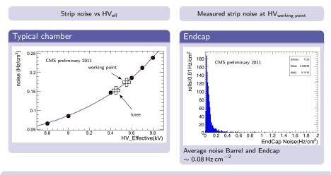
The noise is computed measuring hit rates during periods without beam collisions Most chambers show an intrinsic noise below  $0.5 \,\text{Hz}\,\text{cm}^{-2}$ , negligible for accidentals in the trigger system
