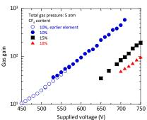
Voltage tolerance is improved and that the element works well at higher gas conditions.
