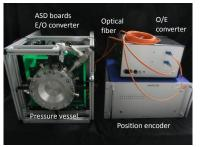
High pressure vessel Inner size: 154 mm\u00f6 x 30 mm<sup>t</sup> Pressure: < 11 atm Helium leakage: < 10<sup>-7</sup> Pa·m<sup>3</sup>/s Conversion gap: 2 cm
