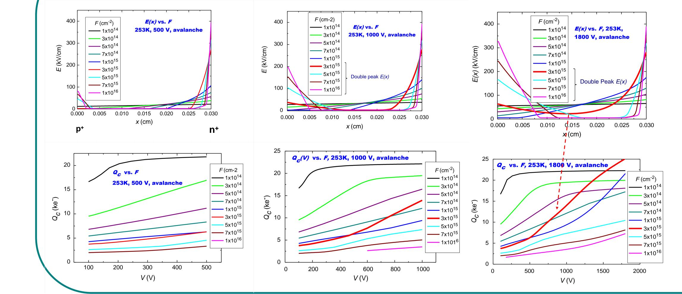
Simulations are carried out for  $F = 3 \times 10^{15}$  cm<sup>-2</sup> at which the experimental collected charge enhancement is maximal.
