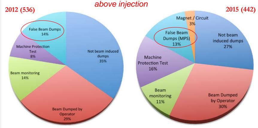
False beam Dumps by Machine Protection Systems stable (LBDS, PIC, BLM, BIC, SIS, QPS, FMCM):
