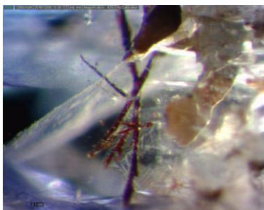
Figure 2a. Ferrocolumbite mineral inclusion (60x magnification).
