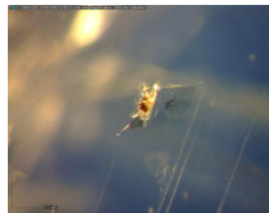
Figure 2b. Rutile mineral inclusion (40x magnification).
