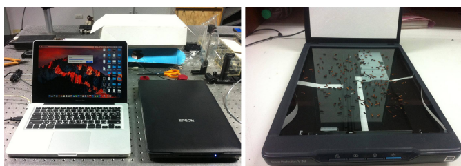
Figure 1. The hardwares used in this work. Images of rice grains are captured by a flatbed scanner. The images are send to a laptop and analyzed via Mathematica software.
