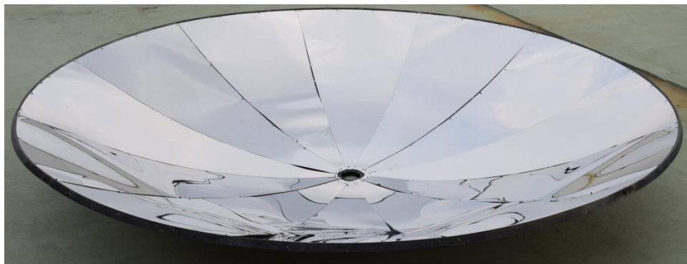
Figure 2. The home-built parabolic mirror for the solar pump laser.
