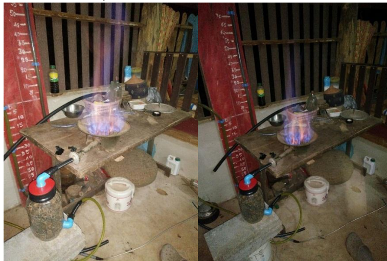
Figure 2. Installation Ferric hydroxide
