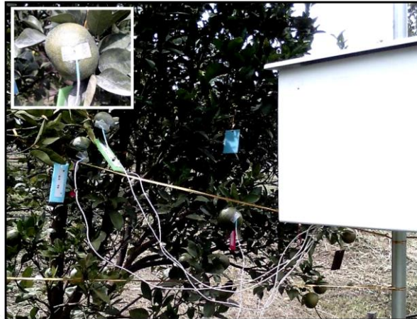
Figure 3. Example of the multi-sensor thermometer used in a mandarin orange cultivation field of the Royal project, located in the northern Thailand. The device is set in a rainproof container (the white box) fixed on a stand with 1 m height. The Inset shows a thermocouple wire attached on the surface of an orange.
