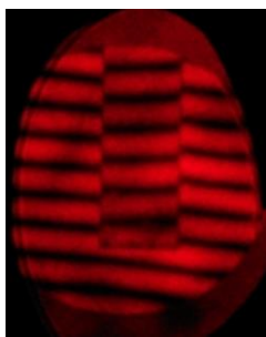
Figure 3a. The fringe pattern on the surface of gauge block and reference flat
