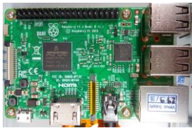
Figure 1a. The Raspberry Pi board for image processing and control camera
