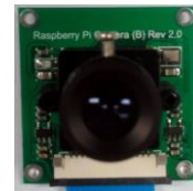
Figure 1b. Raspberry Pi camera for get fringe pattern from system
