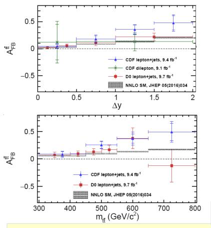
Slope  $\alpha$  of  $A_{FB}^{t\bar{t}} vs \Delta y$  dependence extracted by CDF and D0 compared with SM NNLO predictions
