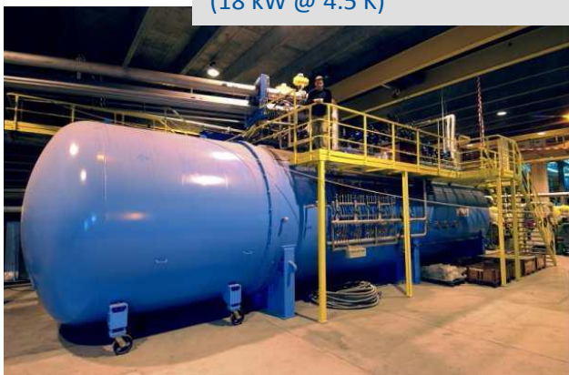
4.5 K refrigerators (18 kW @ 4.5 K)
