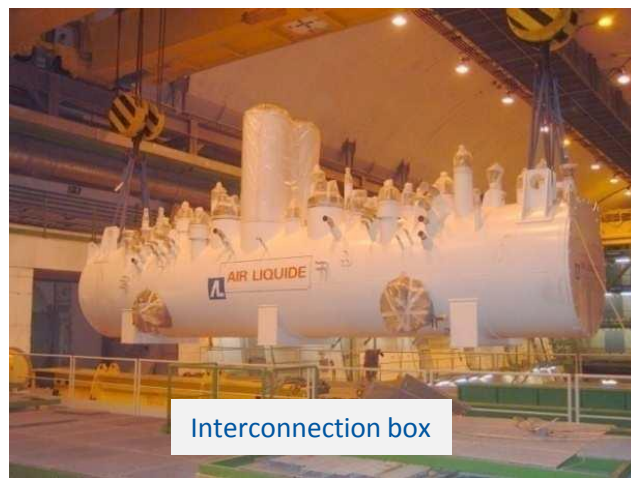
1.8 K refrigeration units (2.4 kW @ 1.8 K)
