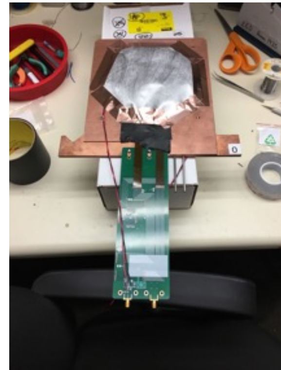
Double layer PCB design and prototype cassette at FNAL
