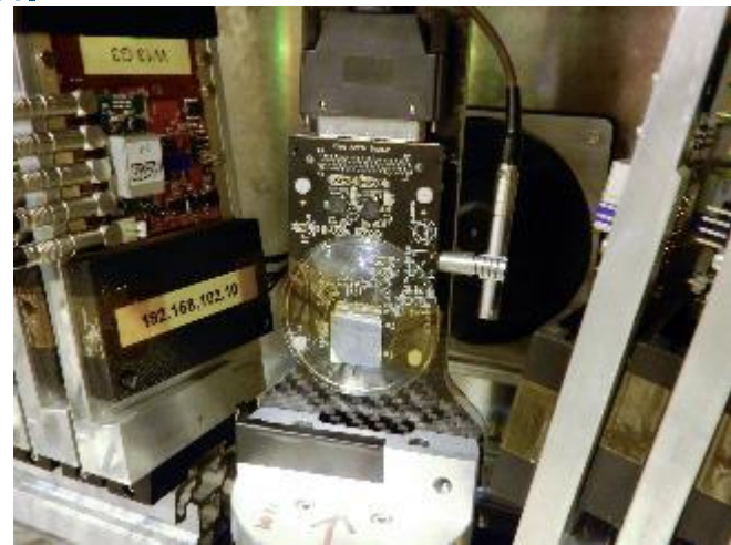
Image of the Timepix3 with a thick silicon layer of 675\mu\text{m} .
