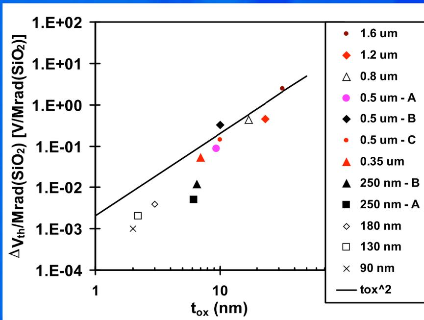
TID-induced threshold voltage shift vs gate oxide thickness.
