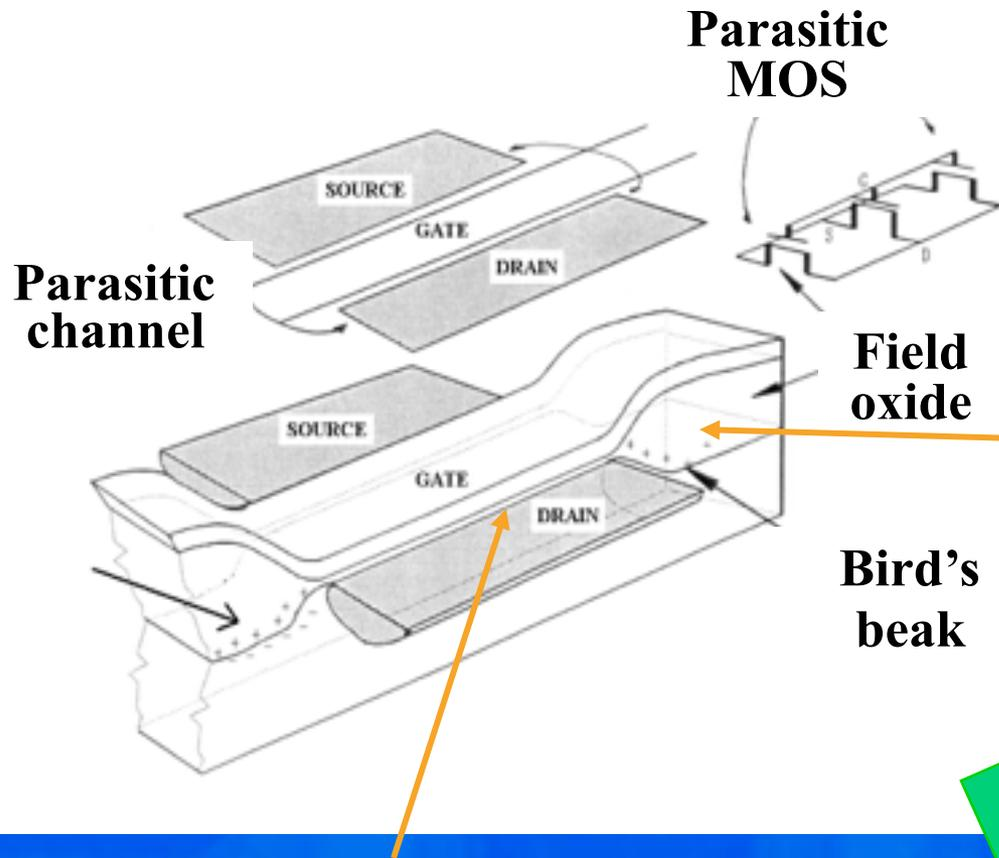
2. Effects in the thick lateral isolation oxide (STI) between source and drain of a transistor
