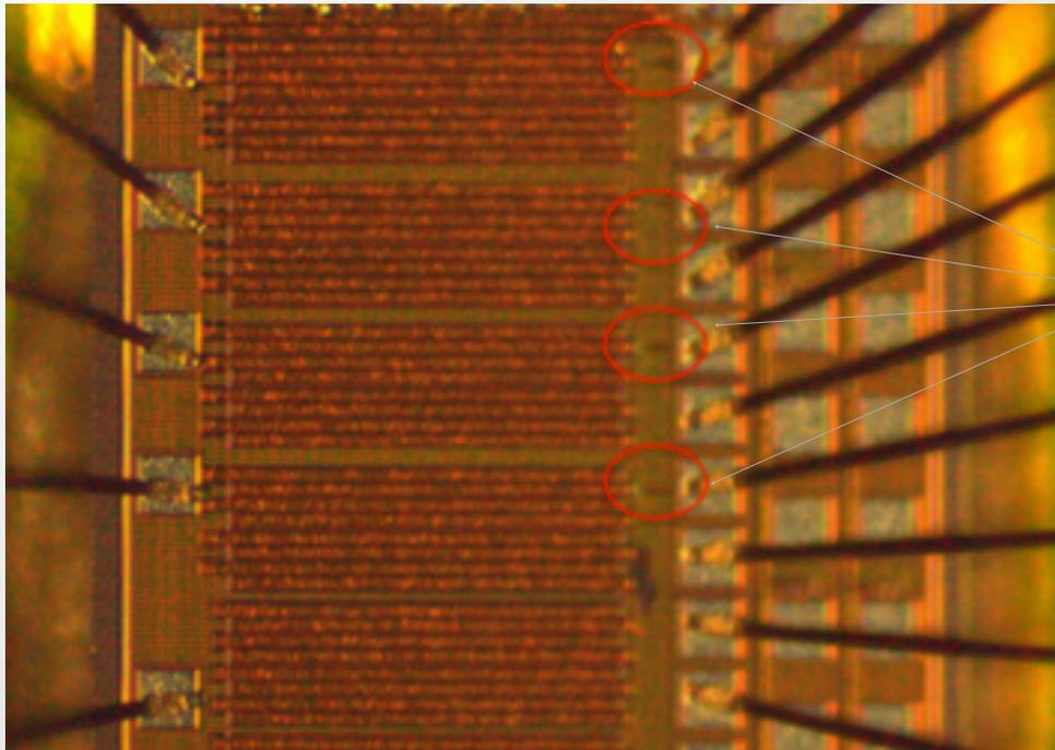
Evidence of SEB on test chips with LDMOS
