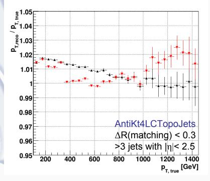
Jet response before (black) and after (red) applying a correction based on multijet bootstrapping
