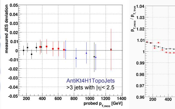
Resulting measurement of the JES, relative to the reference region (colours are used to highlight iterations)
