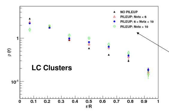
Pile-up events are expected to have multiple vertices and a correlation between the primary vertex multiplicity and shapes is expected:
