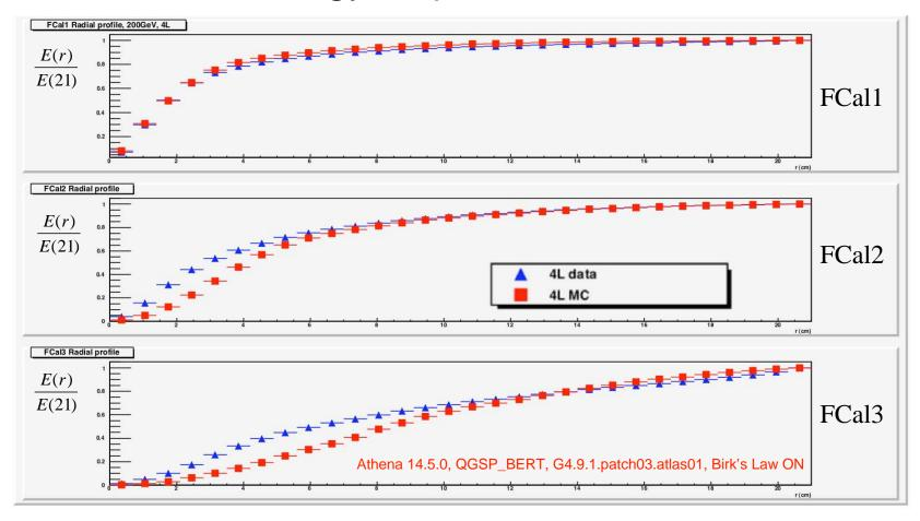
E(r) is the energy within a cylinder of radius r, centred on the beam impact point: 21cm is the limit before reaching the FCal edge (from the 4L or 4H positions).
