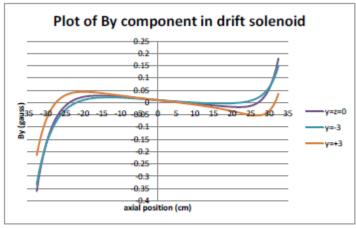
Figure 3.27 Plot By component of the field along the axis of the Drift solenoid (currents in Appendix A).
