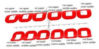
Figure 3.28 Arrangement of the Fine Corrector coils (Y axis)
