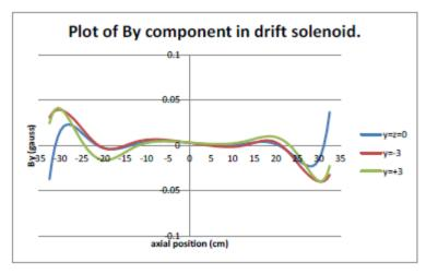
Figure 3.30 Plot of By along drift solenoid with Fine Correction coils in operation
