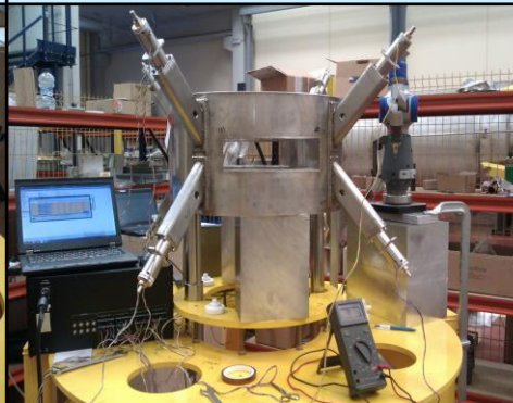
Cryostat and Coil Supports assembled
