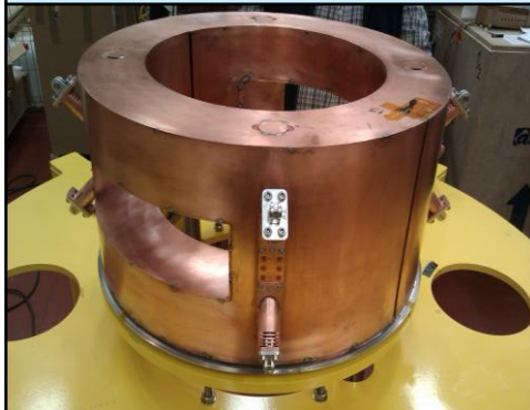
Casing with the Radiation Screen placed around
