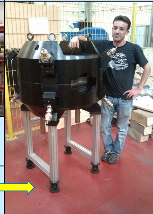
Casing insulated with Superinsulation
