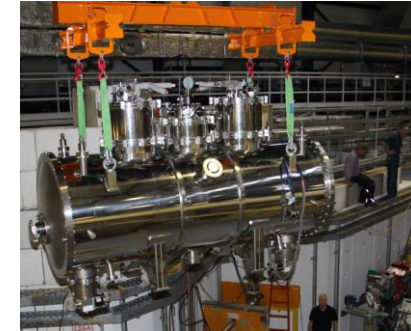
Stripline kicker laboratory tests
