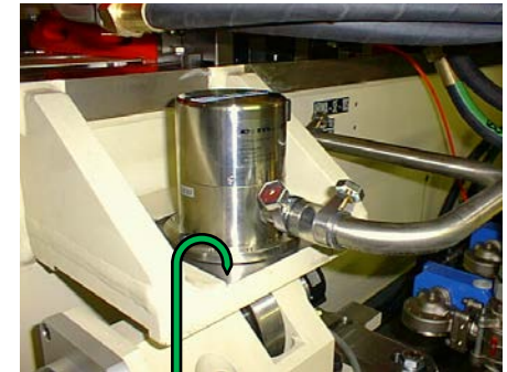
G: +/- 0.002mm grinded support
