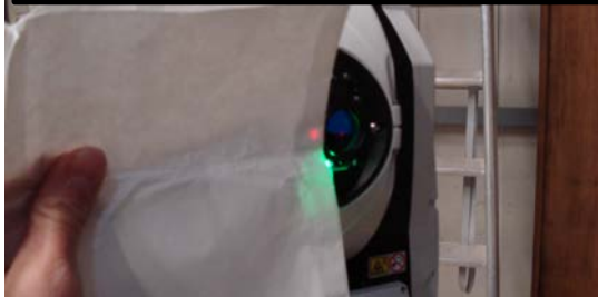
Autocollimation of the laser beam
