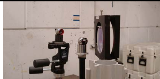
Extreme position (approx. 60°) of the glass window regarding the laser beam
